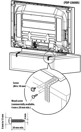
Drill a hole in the middle at the rear of the tabletop panel before using a wood screw. Perform this work the same way on the left and right sides.
