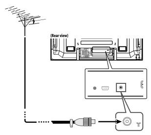
For viewing analogue broadcasts only, connect the 75-ohm coaxial cable (commercially available) to ANT (analogue input) terminal.
