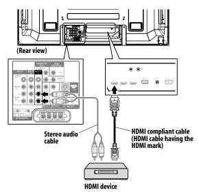
For INPUT 4 and INPUT 5, connect just an HDMI cable - this carries both the audio and video signals.
